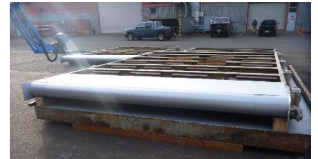
Rounded caps on overflow weirs
